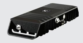
Cel-Fi GO X is optimised for stationary applications such as buildings, factories, warehouses, and similar. It features 100dB of system gain and provides the largest mobile coverage footprint in its category.
