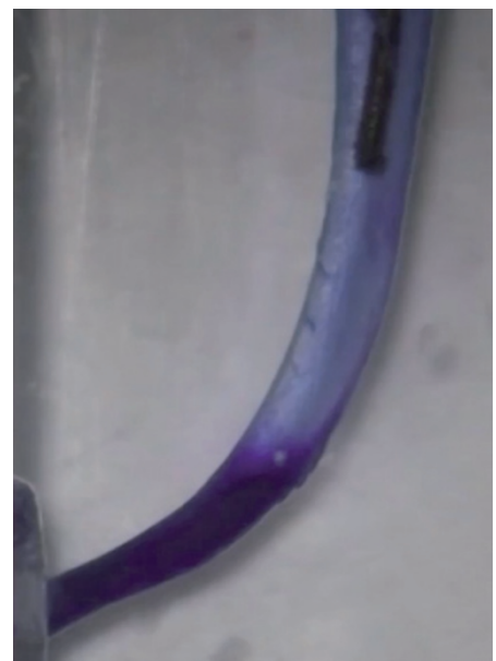
Fig. 4 The clear zone between the open ended needle tip and the apical blue liquid shows the effect of active irrigation beyond the needle tip during a flow rate of ca. 6 ml/min
