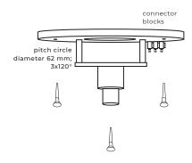
Fix the groundplate with screws to the ceiling.
