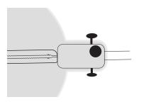
Carefully fix loosely with the supplied knurled-head screw by hand.
