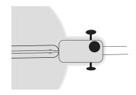
Carefully fix loosely with the supplied knurled-head screw by hand. Do not use a screw-driver. Do not screw too tightly, ensure there is at least 1 mm tolerance between the glass and the screw.
