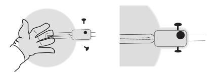
Carefully fix loosely with the supplied knurled-head screw by hand. Do not use a screw-driver. Do not screw too tightly, ensure there is at least 1 mm tolerance between the glass and the screw.
