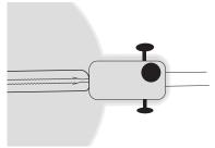
Carefully fix loosely with the supplied knurled-head screw by hand.
