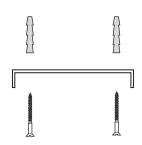
Affix the bracket to the ceiling with 2 screws (hole size max. 4.5 mm, 50 mm apart).
