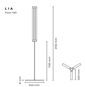
Туре Floor light Brass Material Environment Indoors 540 x 2150 mm Dimensions Cable Length 1500 mm Weight 3 kg Certification IP20 CE EU/UK 230 V
