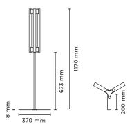
Floor light Туре Material Brass Environment Indoors 370 x 1170 mm Dimensions 1500 mm Cable Length Weight 2.4 kg Certification IP20 CE EU/UK 230 V
