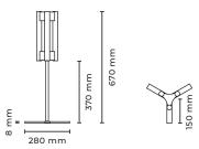
Floor light Type Material Environment Indoors Dimension 280 x 670 mm Cable Length 1500 mm Weight 2.2 kg Certification IP20 CE EU/UK 230 V Lamps max. 3 x 35 W, S14s
