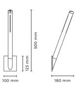
Туре Wall luminaire Material Solid brass and glass
