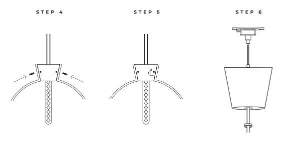
Fix loosely all the supplied screws by hand into position. Do not use a screwdriver.
