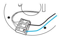
Thread the cables through the ball joint and screw the stem into the ball joint. After that connect the cable with the clamp on the groundplate.
