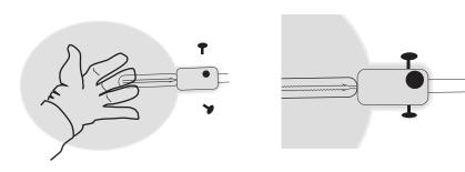
Carefully fix loosely with the supplied knurled-head screw by hand. Do not use a screw-driver. Do not screw too tightly, ensure there is at least 1 mm tolerance between the glass and the screw.
