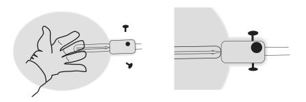
Carefully fix loosely with the supplied knurled-head screw by hand. Do not use a screw-driver. Do not screw too tightly, ensure there is at least 1 mm tolerance between the glass and the screw.
