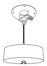
The cables only come out of one stem. This can simply be screwed on.
