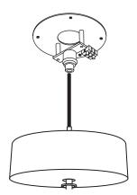
The cables only come out of one stem. The others can simply be screwed on.
