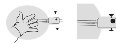
Carefully fix loosely with the supplied knurled-head screw by hand. Do not use a screw-driver. Do not screw too tightly, ensure there is at least 1 mm tolerance between the glass and the screw.
