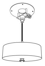
The cables only come out of one stem. The others can simply be screwed on.
