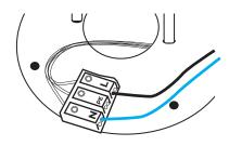
Thread the cables through the ball joint and screw the stem into the ball joint. After that connect the cable with the clamp on the groundplate.
