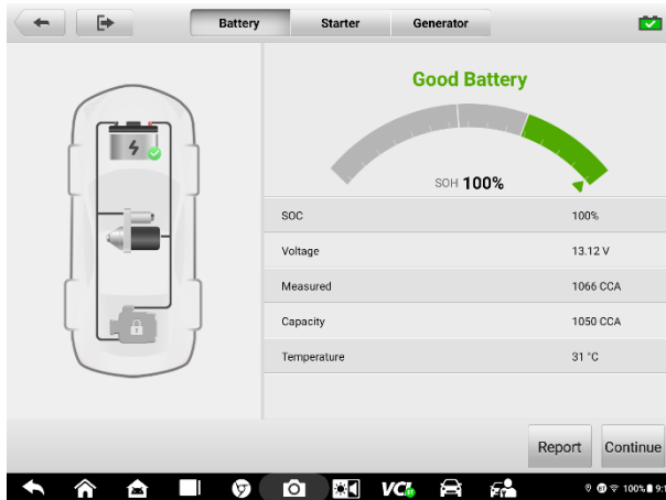
Figure 11-6 Battery Test Results Screen
