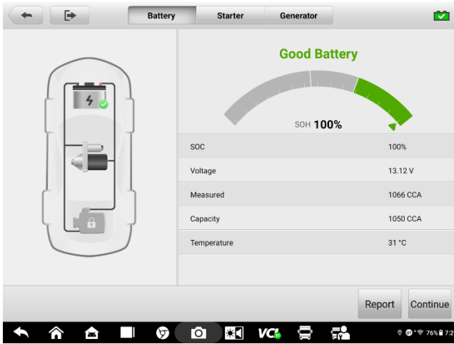
Figure 17-7 Battery Test Results Screen
