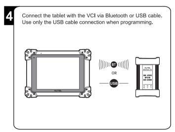
When the VCI device is properly connected to the vehicle and the tablet, the VCI status button on the bottom tool bar of the screen shows a green badge, indicating the platform is ready to start vehicle diagnosis.
