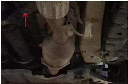
4) Once the factory bolt is removed install the front mounting tab. Place the M10 carriage bolt into the frame tab. (Fixing it with tape is recommended to keep the bolt from coming out of the tab during installation) Install bolt and tab into the frame as shown.
