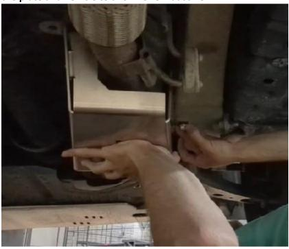
6) Reinstall the factory removed bolt at the rear of the plate and tighten.
