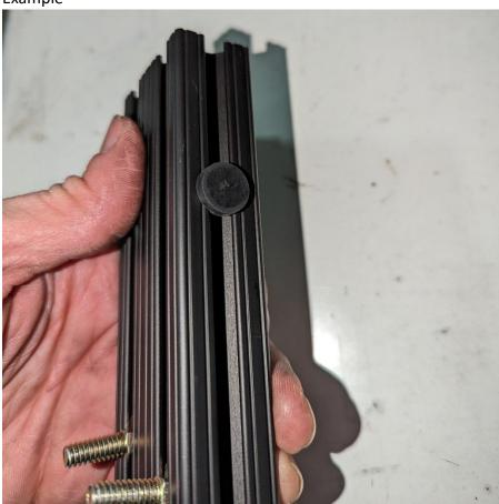
Install cross member at the front most crossmember space on the side rail. Placing the rubber bumpers forward with the  $\frac{1}{2}$ -20 carriage bolts pointing downward. Line up the  $\frac{1}{2}$ -20 bolts with the stiffener.
