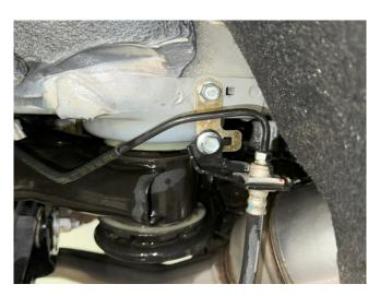
Step 7. Support driver side rear lower control arm with a floor jack.
