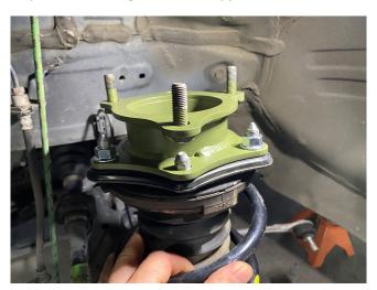
Step 15. Reinstall front strut and knuckle in reverse order. Use OEM nuts to secure the strut to body. Torque upper mounting nuts to 25 ft-lb. Strut pinch bolt to 88 ft-lb. brake caliper bolts 91 Ft. Lb.
