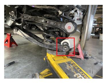
Step 12. Carefully lower jack to release pressure on spring, remove spring.
