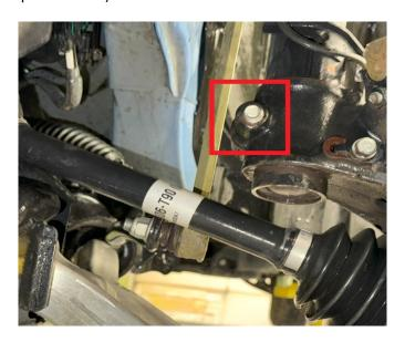
Step 11. Remove lower ball joint nut and using a heavy hammer, strike lower arm to carefully unseat lower ball joint from bottom of knuckle.
