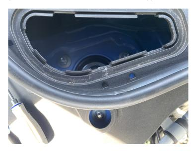
Step 2. Remove nuts holding struts to body, leave one nut on so struts do not fall when lifting vehicle to access bottom bolts.
