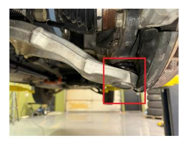
Step 12. The knuckle should slide free from strut.
