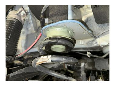
Step 15. Using floor jack or screw jack, lift lower control arm until bolt holes line up.
