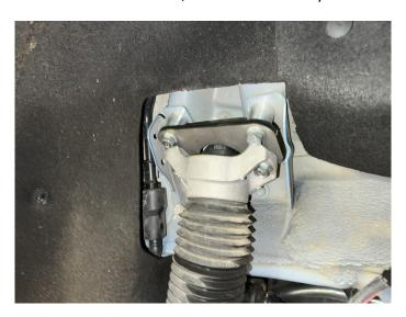
Step 11. Remove bolt holding lower control arm to wheel hub as shown:
