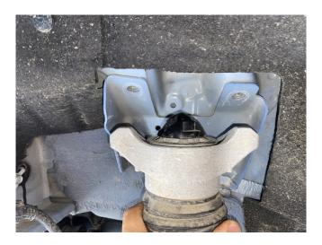
Step 9. Bolt shock to shock bracket using hardware provided in the kit. Tighten bolts to 35 ft-lb.
