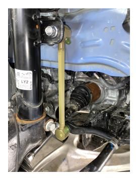
Step 17. Install BLBL on brake line mount, to relocate brake line brackets. (see photo)
