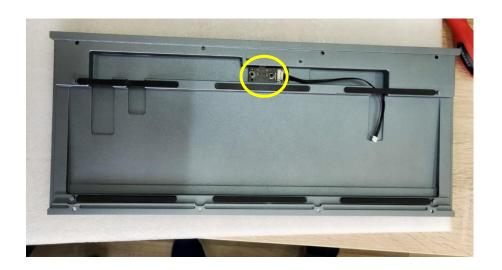
Place the brass standoffs at the marked locations in the picture below and secure them in position by screwing in six pieces of brass standoffs from the front of the mounting plate. Utilize the included flat-head screws found in the zip bag for this process.將銅柱放置在下方圖片中標記的位置,並使用夾鏈袋中附帶的平頭螺絲從定位板的正面將六個黃銅支架固定在位。
