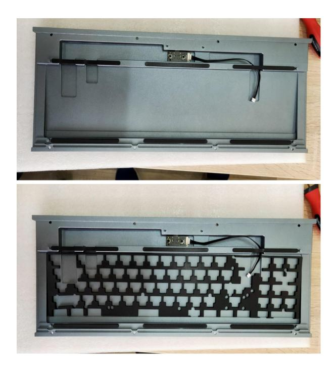
Connect the main PCB with the daughterboard and attach the ffc to the F-row. Place the top case and secure it with M2 black screw\* 8 pcs to complete the assembly. 最後,將主 PCB 與子板連接,並將排線接上 F 排。蓋上上蓋並用 8 顆 M2 黑色螺絲固定,組裝完成。
