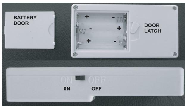
1. Place 3AA batteries inside the battery compartment with the polarity as shown.
