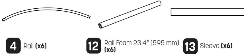
Insert a rail foam **(12)** into a sleeve **(13)**. Then insert a rail **(4)** into the foam you just placed inside the sleeve.
