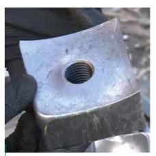
Bolt on cutting teeth Can be rotated to maximise wear part life Tight tolerance cutting action
