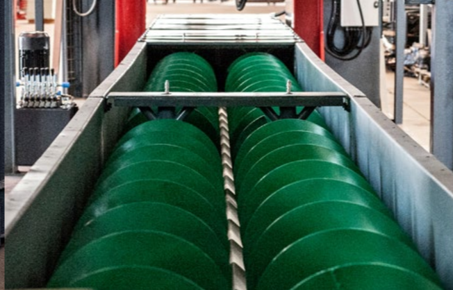
Screws to carry out the dry mud
