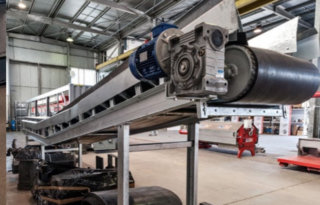
Belt to collect and convey the mud cakes
