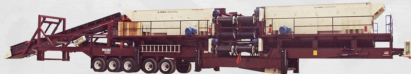
Masaba Portable 70 Ton Surge Bin w/ Brute run-on jacks, vibrating pan feeder, and folding 72" end discharge conveyor.
