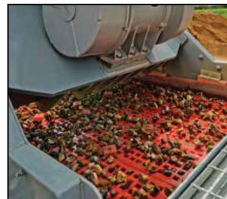
Washed scrubbed aggregate
