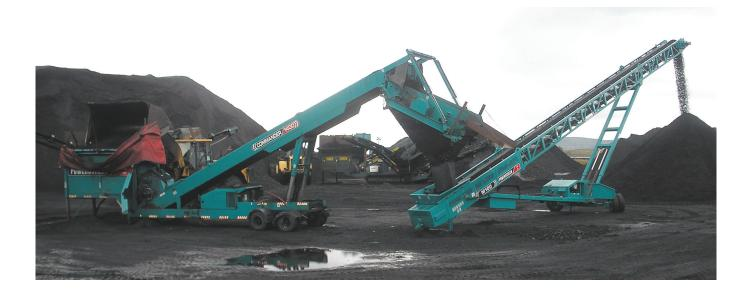
The Powerscreen® Commander 1400 is a high capacity mobile screen that has been engineered for quick installation and ease of relocation making it ideal for applications including topsoil, coal, crushed stone, recycling, sand and gravel.
