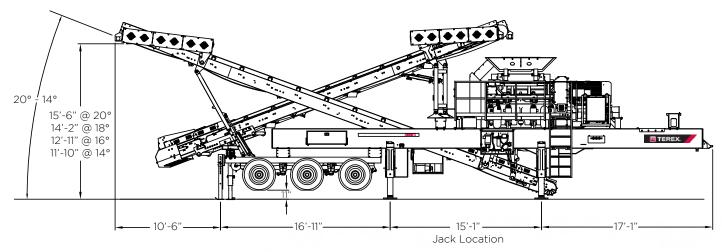
Note: All drawings shown with optional overflow chute, switchgear and run-on jacks
