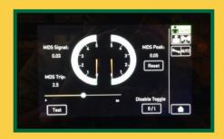
A problem for any industrial grinder has to do with tramp metal entering the hog box and causing significant damage, which leads to downtime. The Metal Detection System<sup>TM</sup> (MDS) engages within milliseconds whenever the grinder's rotor makes contact with tramp metal.
