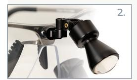
Slide the headlight onto the frame until fully seated. Align the frame mount to the channel mount on the RX Insert and slide downward onto the screws. Insert should set behind nosepads.
