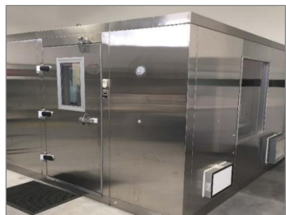
Figure 2: Stainless Steel Bioaerosol Test Chamber used for all M40 Testing. Chamber is equipped with HEPA in/out, multiple bioaerosol sampling ports, decontamination and pressure balance. Exterior picture.
