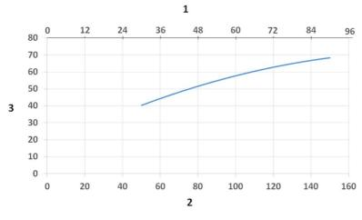
Sound Level diagram: 1) X- Axis: Air Flow Rate (cfm) 2) X- Axis: Air Flow Rate (m/h)
