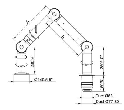
Part number: 70600344 Max. working radius: 630 mm (24,8 in) A: 400 mm (15,7 in) B: -
