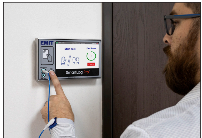
Figure 24. Performing a single-wire wrist strap test
