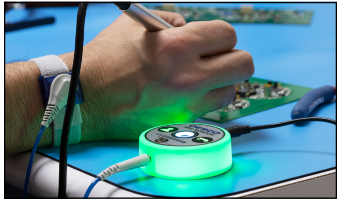
Figure 8. Illuminating green to indicate a proper operator path-to-ground
