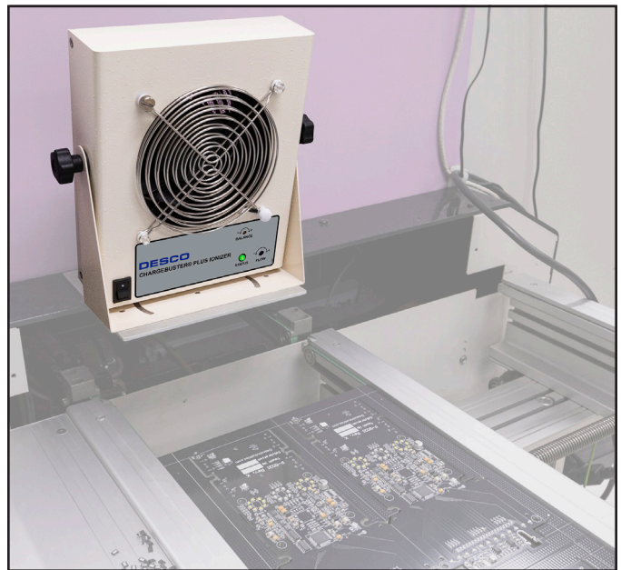
Figure 7. Using the Chargebuster Plus Single-fan Ionizer at a machine station
