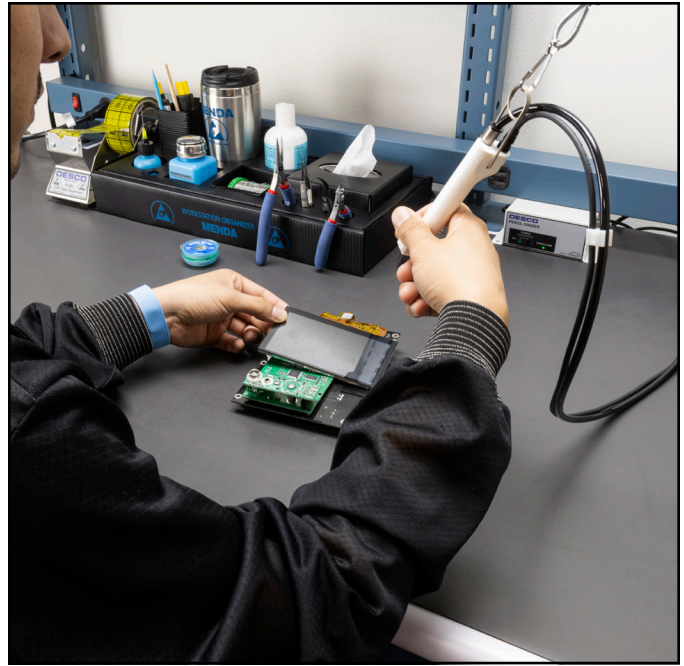
Figure 7. Using the Pencil Type Ionizer
