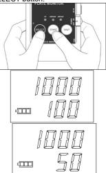
4. Point the plate in the airflow of the ionizer to be measured and press the START button.
