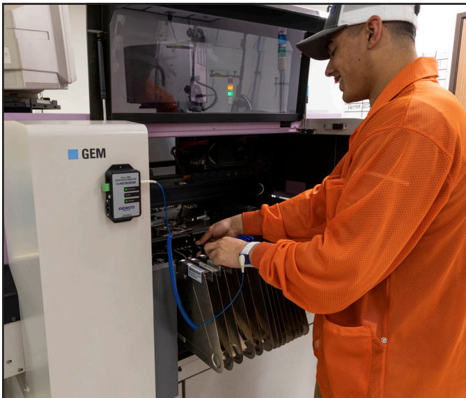
Figure 15. Using the Full-Time Continuous Monitor at a machine station
