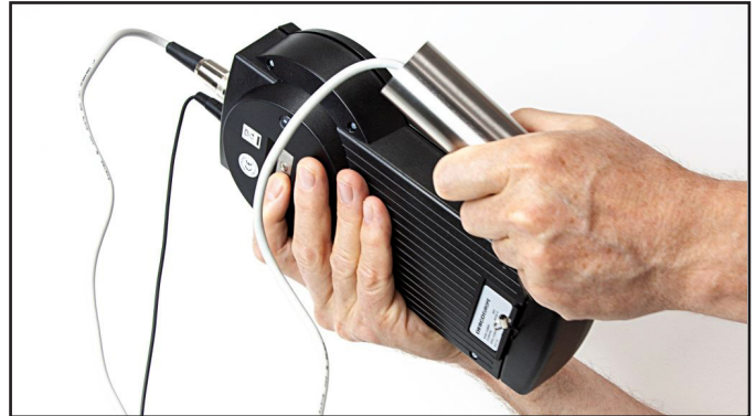
Figure 4. Momentarily touching the ground touch plate to ground the operator
