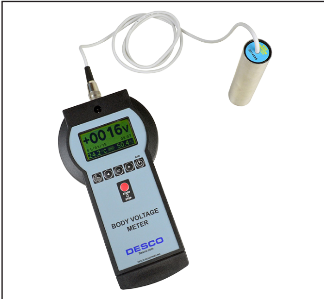
Figure 1. Desco 19431 Body Voltage Meter
