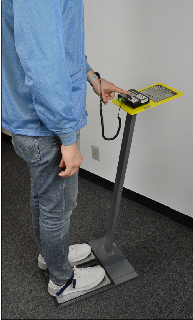
Figure 13. Using the 19271 Combo Tester X3 with Stand
