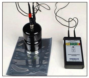
Figure 4. Using the Concentric Ring Probe with the Desco Surface Resistance Checker
