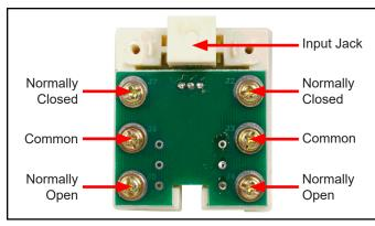
Figure 5. Full-Time Continuous Monitor Relay Box features and components
