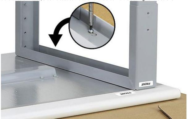
**4.** The front of the legs have 1/4" holes. The back side of each leg has 4 smaller, threaded holes. Position the back bar over the threaded holes, insert screws and tighten. (There are no lock washers or nuts required here)
