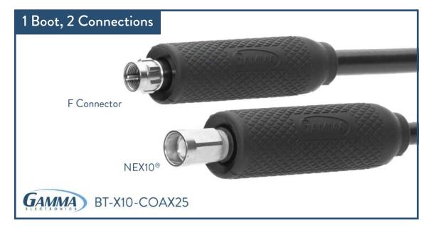
Gamma's NEX10 & F Connector Weatherproof Boot is an IP68 rated boot that works on both NEX10 and F Connections. It typically comes pre-installed on the cable allowing it to slide up and over the connection creating a watertight seal. As part of the IP68 testing process the boot has been placed in water tanks more than 1 meter in depth for over 30 min without showing any signs of water ingress.
