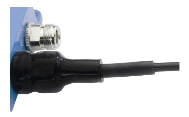
We took LMR 195 and added a unique heat shrink that builds up the outer diameter of the cable right at the junction of the connector and the cable. Why? Because Cold Shrink can shrink to really small sizes, but not quite LMR 195 small.
