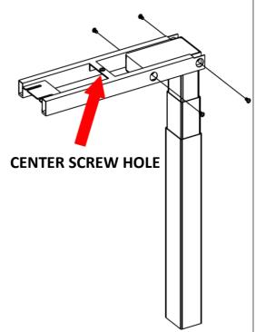
Insert the Side Bracket (Part 4) into the End Frame (Part 1) and align the screw holes as shown.
