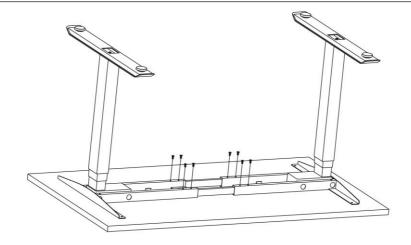
Ensure the Cross Rails (Part 2) are positioned evenly within the End Frames (Part 1). Insert and fasten using 8 screws from Pack E in a criss-cross pattern to fix the Cross Rails in position.
