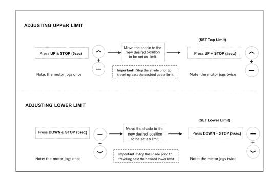
!!WARNING!! - Move shade in short increments by pressing the UP/DOWN button in 1 second intervals (pressing the UP/DOWN button for more than 3 seconds may send the shade past desired upper/lower limit and may result in damage to the product). Once you have reached the desired upper/lower limit, you can adjust the limit with either the UP and DOWN buttons. (remember to adjust in short increments!)
