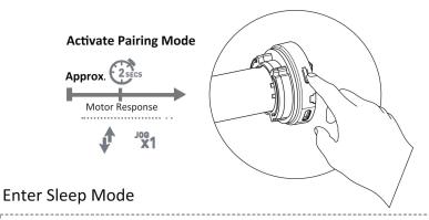
If required, to place the motor back into "Sleep Mode" press and hold the programming button for a period of 10 seconds. Release the button when the motor has jogged **three times**. The "Sleep Mode" has been activated.
