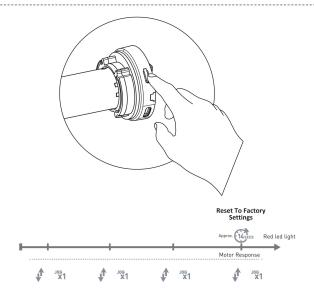
The motor will jog 4 times before the reset is complete. The programming button must be held the entire time. Red led light on confirm the factory reset is complete.
