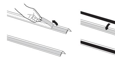
3. Stick the 2 Magnetic strip on each side of the window inside frame
