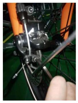
Step 4: After Unscrewing the two bolts and then hold the brake by hand, so that the position of the brake pad and disc brake disc can be corrected.
