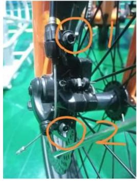
Step 2: Unscrew the first bolt anticlockwise with an Allen wrench (rotate it for about 3 turns).
