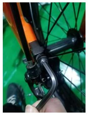
Step 3: Unscrew the second bolt anticlockwise with an Allen wrench (rotate it for about 3 turns)
