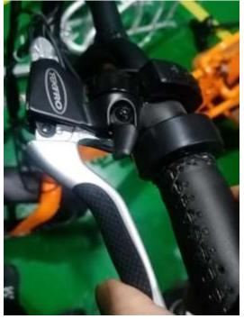
Step 5: Tighten the first bolt clockwise with an Allen wrench. (You still need to hold the brake at this time)
