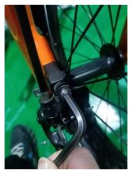
Step 6: Tighten the second bolt clockwise with an Allen wrench. (You still need to hold the brake at this time)
