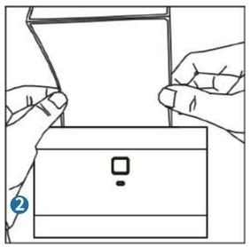
Adjust the width of paper guide, insert paper from back. The label will be positioned at the tear-off point. Jadens is ready to print.
