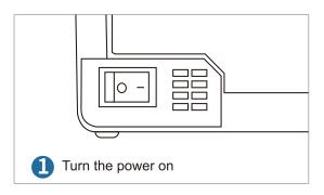
Switch on the printer and wait 7 seconds for the printer to initialize.
